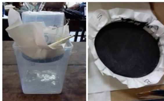
Figure 1: The simple filtration apparatus (left) and the micro-sized carbon material from coconut shell leftovers (right).
